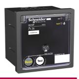
Residual current protection relay, VigiPacT RH10P, 300mA, 12/24VAC 50/60Hz, 12/48VDC, front panel mounting
