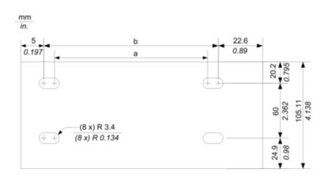
**NOTE:** You can use M4, M5, M6, or UNC #6 screws in the fastening holes.
