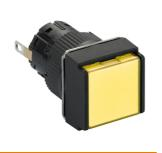
Monolithic pilot light, Harmony XB6E, square Ø 16, IP65, yellow, integral LED 24VDCpolarised, connector
